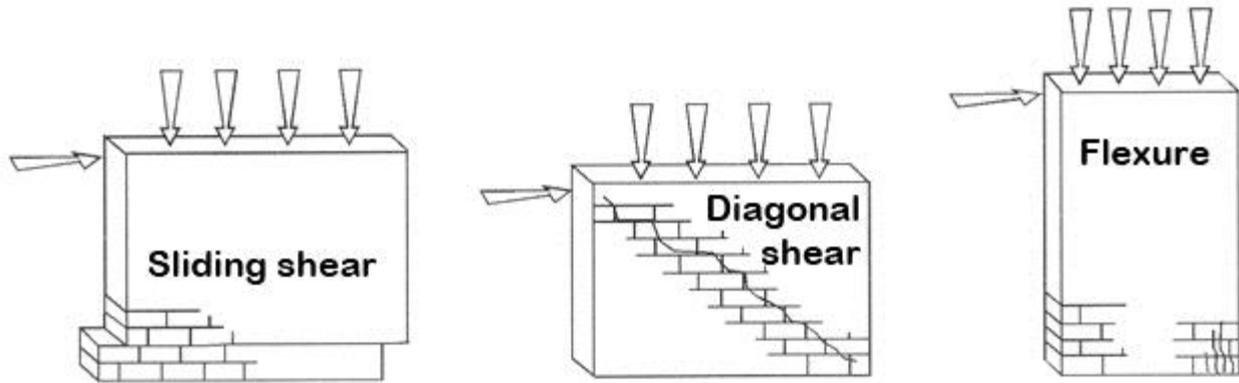
**Fig. 1.1.1.** Resistant mechanism of masonry walls [1]
