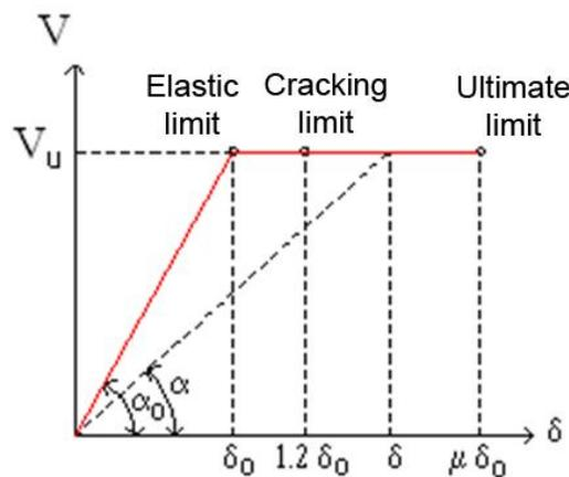
**Fig. 1.5.1.** Shear-displacement diagram of a single pier
