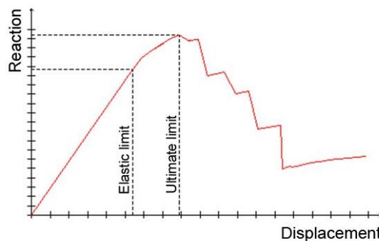
**Fig. 1.5.2.** Shear-Displacement diagram
