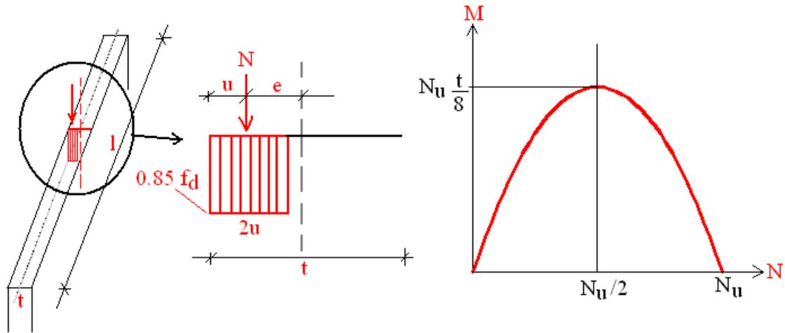
**Fig. 1.6.7.** Ultimate moment for out-of-plane flexure
