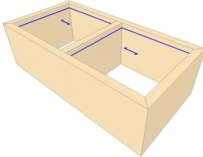
**Fig. 1.1.3.** Box behavior of masonry structure
