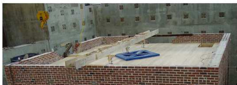
Figure 7.2. The tested roof diaphragm
