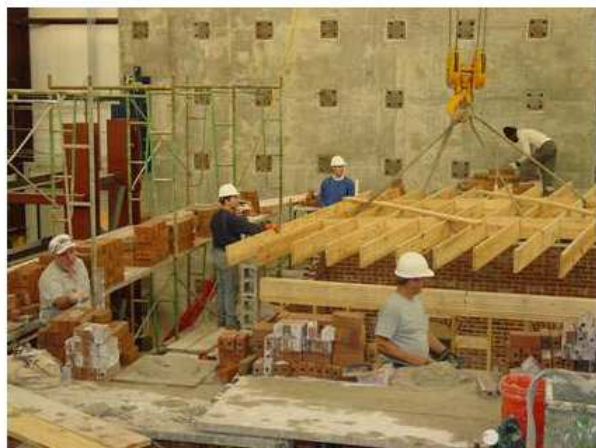
Figure 6.17. Assembly of the floor systems
