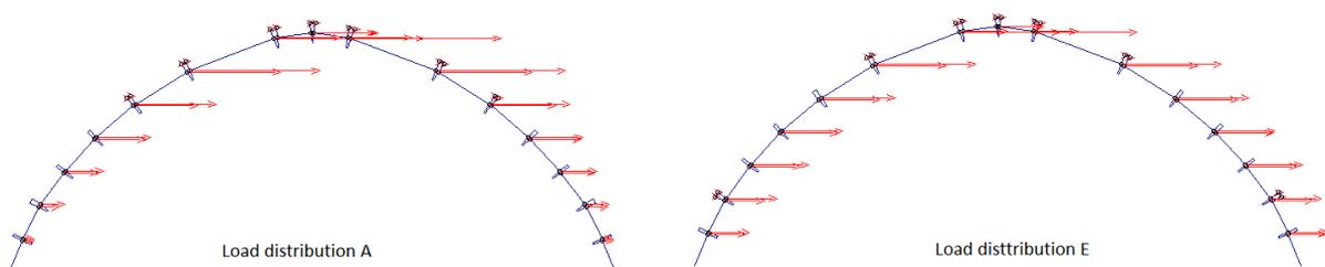
Figure 15. Load distributions in nonlinear static analysis
