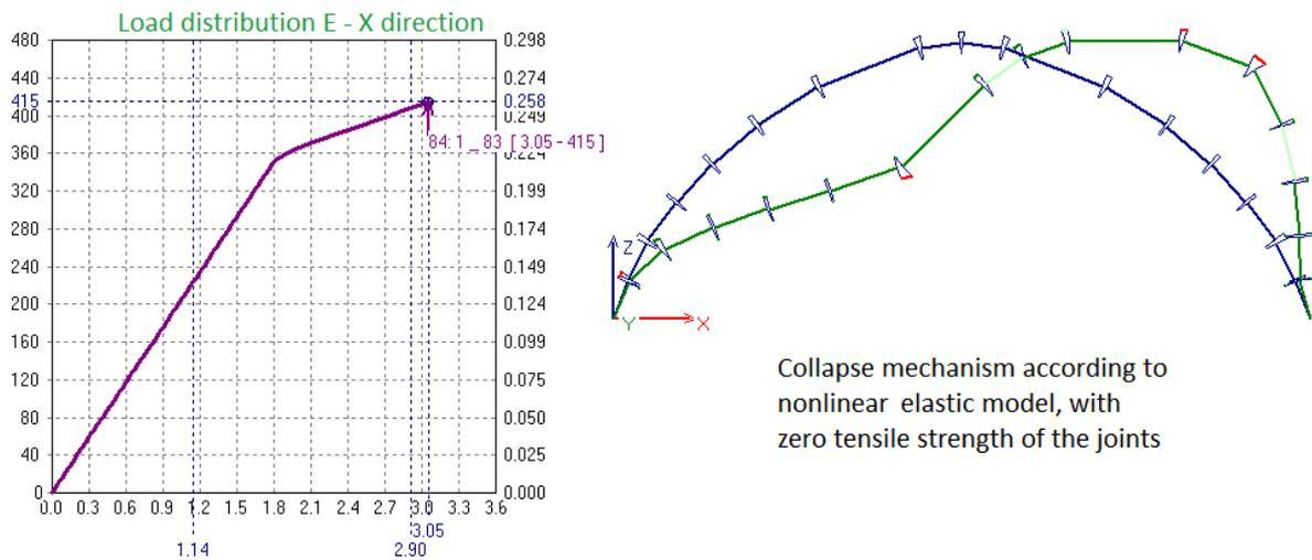
Figure 16. Nonlinear static analysis with zero tensile strength
