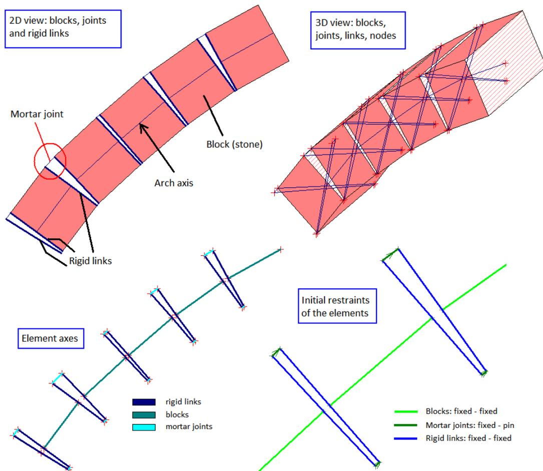
Figure 2. The finite element model block-joint
