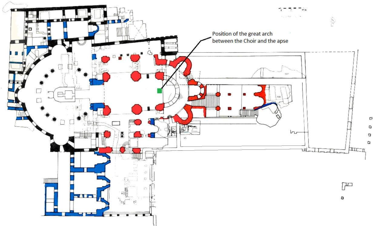
Figure 3. Floor plan of the monument: Constantinian period (4<sup>th</sup> century) in black, restoration of Constantine Monomachos (11<sup>th</sup> century) in blue, structures built by the Crusaders (12<sup>th</sup> century) in red.
