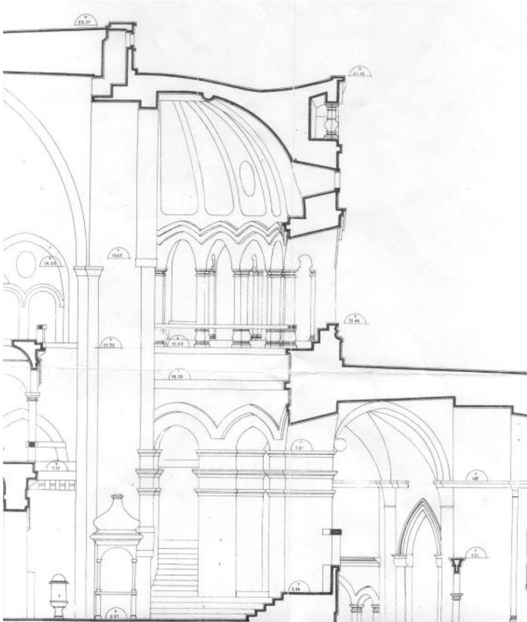
Figure 4. Vertical section of the apse
