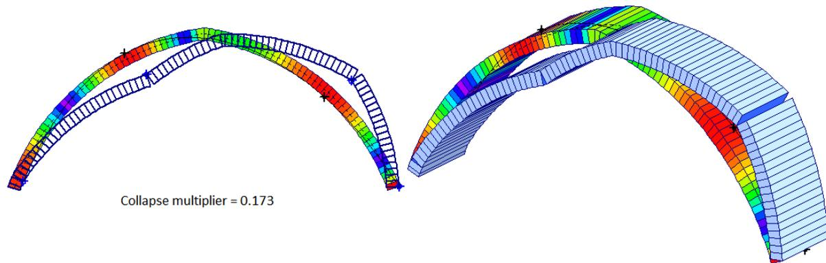
Figure 11. Collapse mechanism for seismic action
