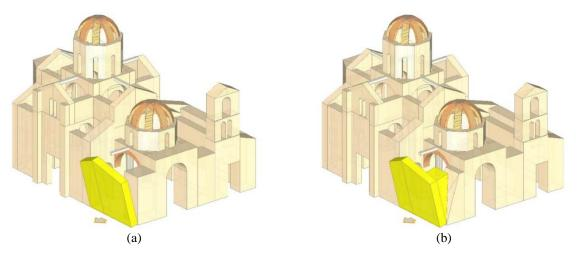
Figure 5: a) M05 - Overturning of a north wall; b) M06 - Overturning of a north wall wide one side wing.
