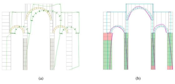
Figure 8: Pushover analysis, last step: a) displacements; b) Thrust-lines and verifications.
