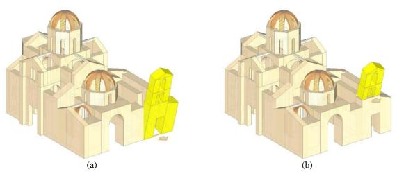
Figure 3: a) M01 - Overturning of the belfry façade; b) M02 - Overturning of the belfry.
